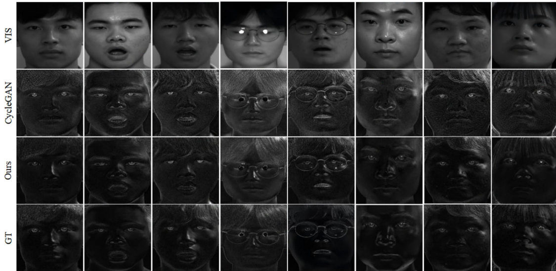
Fig. 6. Comparison with CycleGAN-generated results. The first row shows the VIS modality, the second row shows the results generated using CycleGAN, the third row shows the results generated by our FC-Net, and the last row shows the real acquired polar image.
