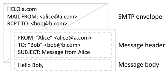
Figure 1: Example SMTP headers in a transmission (inspired by Figure 3 in Chen et al. [5]).
