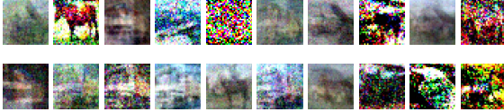
Figure 3: Directly Extracted Data under DDP. Rescaled clipped and noised gradients from a mini-batch with 20 data points from CIFAR10 dataset. DDP setup: c = 1 , \sigma = 0.1 , and M = 100 .
