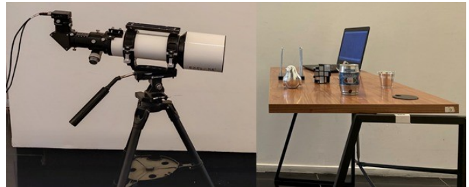
Fig. 1: A photodiode is mounted on a telescope (left) and directed at a shiny object on a desk (right). The photodiode is used to obtain optical measurements from the light reflected from the shiny object’s minuscule vibrations induced by sound.
