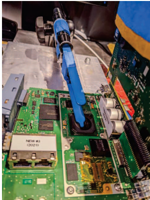
Fig. 9. A stack of two near-field probes, used for observing electromagnetic emanations, can be seen placed on top of Siemens S7-1500 PLC main SoC. Using this setup, CPU bond emanations during the bootup process can be observed.
