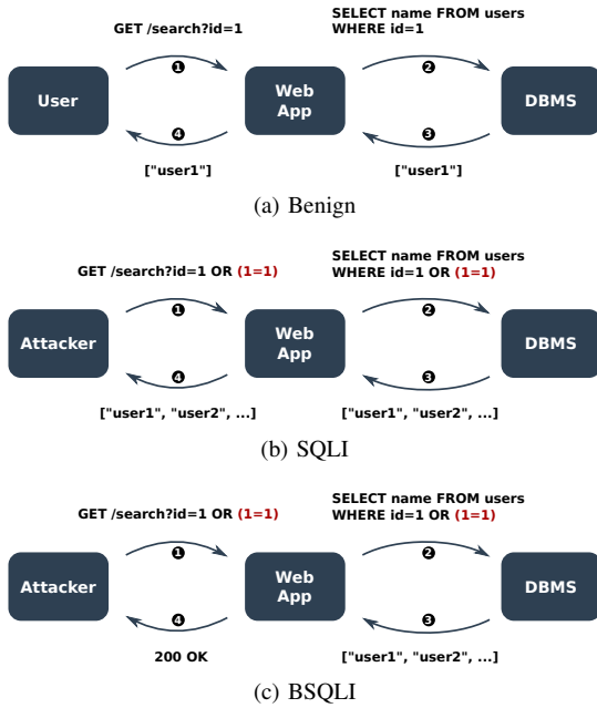
Fig. 1. An illustrative example showing a benign interaction with a web application as well as SQLi and BSQli attacks.
