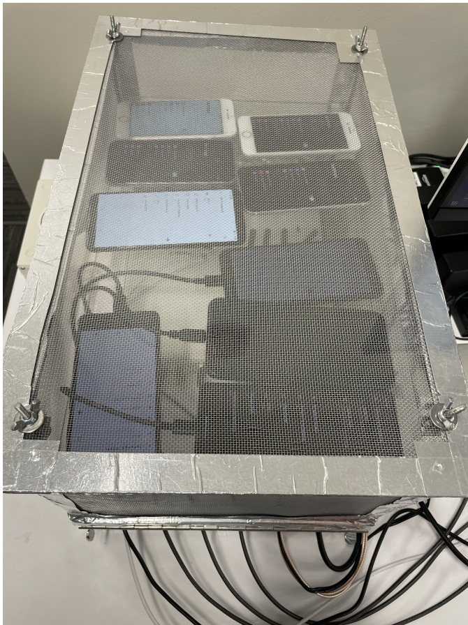
Figure 2. Faraday cage for our active LTE experiments.
