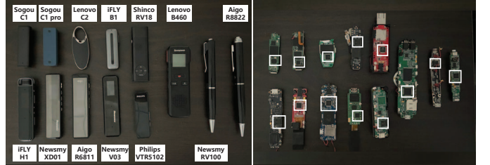
Fig. 11. The appearance (left) and internal PCB circuit (right) of 13 chosen recorders, the label applies to both figures. We use the white boxes to indicate the positions of MSOCs.
