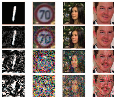
Fig. 6: Original images (first row), AEs with 1 times perturbation (second row), AEs with 5 times perturbation (third row), and AEs with 10 times perturbation (last row)
