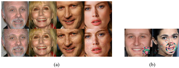
Fig. 9: A verification sample is generally created from an original example by adding a trigger or pixel perturbation in existing works. Such pixel-level patterns can be distinguished by human perception. (a) Sensitive Samples [8] for private verification of model integrity (Second row). The first row is the original images. (b) Triggers (Trojan Square and Trojan Watermark) used in Backdoor attacks [6].
