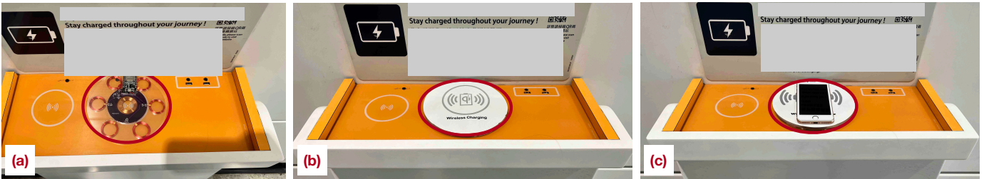
Fig. 32: ParasiteAttack in a subway station. (a) the public wireless charger stuck with a parasite label; (b) the wireless and the parasite label with a signboard cover-up; (c) a victim is using the parasite label to charge his smartphone.
