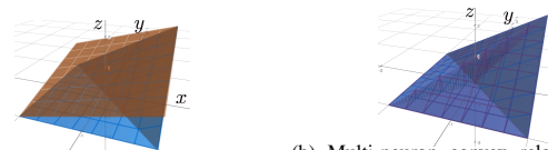
Fig. 7. Comparison of convex relaxation for z = \text{ReLU}(x + y) (shown as bottom blue surface in (a)), where x, y \in [-1, 1] . Vertical axis is the z -axis.
