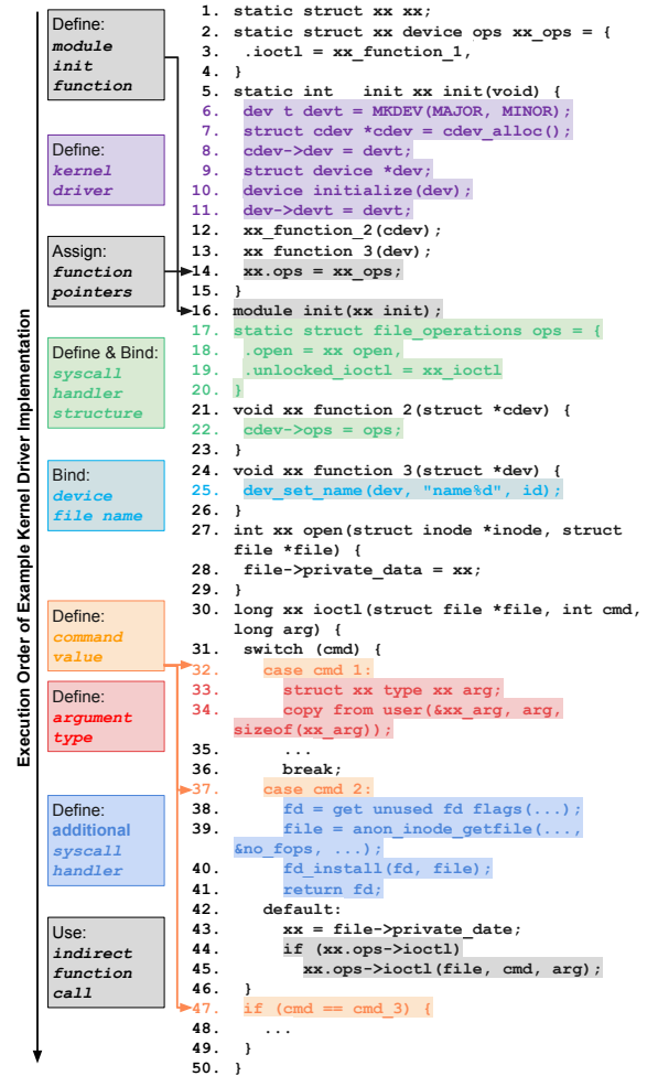
Figure 2: Simplified example kernel driver implementation
