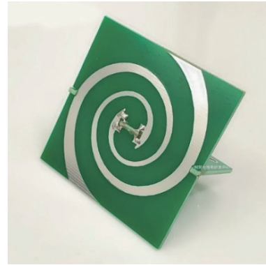
Figure 17 Printed differential antenna for UWB radio.
