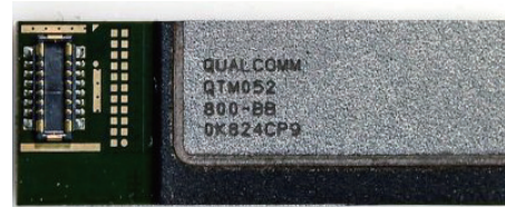
Figure 18 Differential dipole antenna array in an AiP for 5G NR at 28 GHz.
