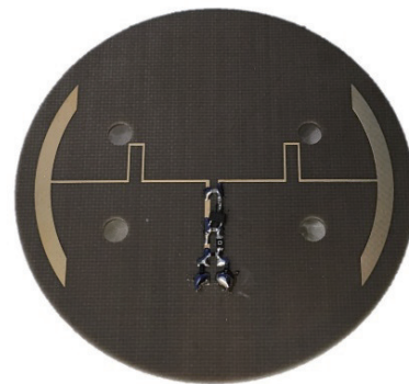
Figure 27 Differential dipole antenna for IoT device.
