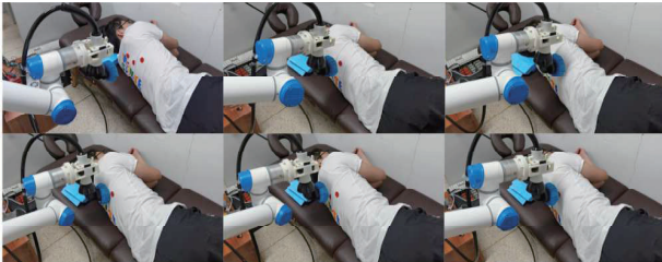
Figure 16. Flow chart of the robot performing a back-slap sputum excretion operation.
