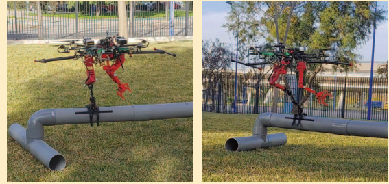
Figure 14. Two snapshots showing experiments with the PBS of the manipulator using the position given by the docking tool.
