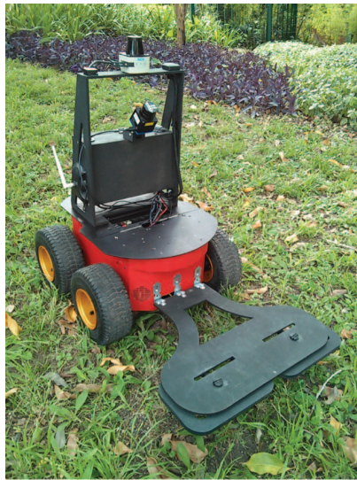
Figure 1. The HRATC 2017 robot platform and sensor suite.
