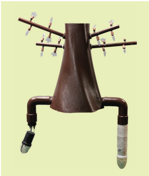
Figure 4. A prototype of the PLANTOID robot. The figure shows two functional roots, a trunk containing a microcontroller main board and a spool of the material used to grow the robotic root in polypropylene (nominal diameter d = 2.5 mm), and an aerial portion with branches that include polymeric artificial leaves (based on controllable hygromorphic plant-inspired material moving in response to humidity, see [39]).
