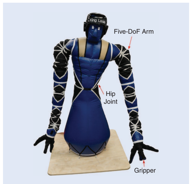
Figure 1. A 14-DoF soft robot named King Louie with no rigid internal structure.
