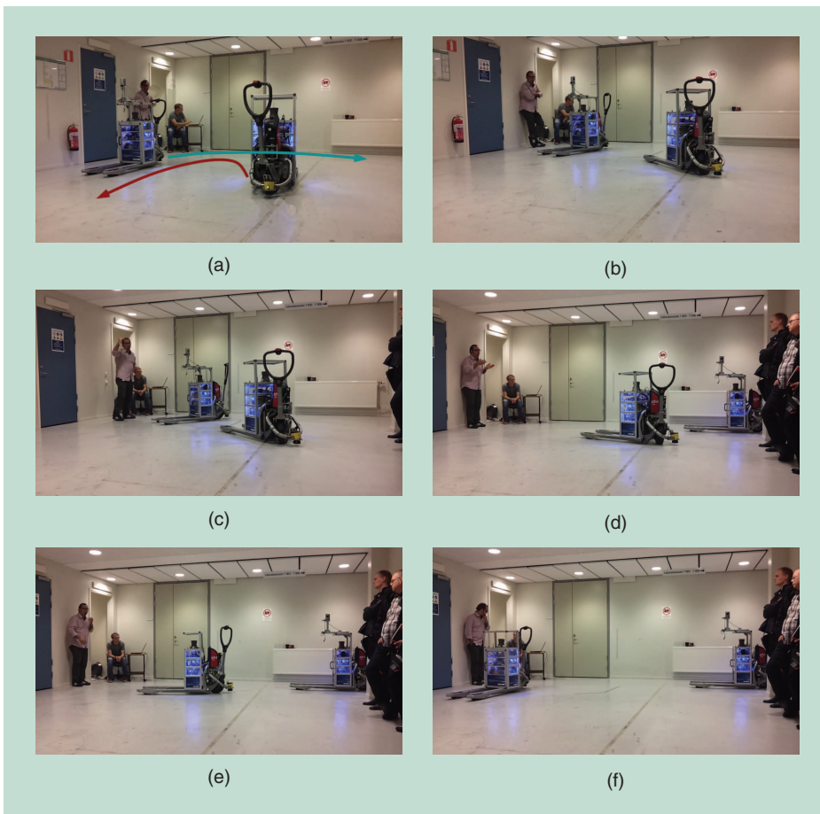
Figure 6. The first scenario: (a) vehicles 1 and 2 and their targets, (b) vehicle 1 is braked, causing vehicle 2 to yield, (c) the brake is released and vehicle 1 resumes motion, (d) vehicle 2 resumes motion, and (e) vehicle 1 and (f) vehicle 2 reach their final poses. (Photos courtesy of Ola B. Pettersson.)
