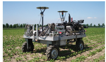
Figure 3. The Intelligent Autonomous Weeder, a robot that performs autonomous weeding operations in arable farming. (Photo courtesy of Wageningen University & Research Centre, The Netherlands.)
