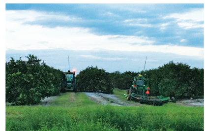
Figure 4. Two autonomous tractors spraying a commercial orange grove. Their activities are coordinated by a high-level supervision architecture. (Photo courtesy of National Robotics Engineering Center and Deere & Company, United States.)
