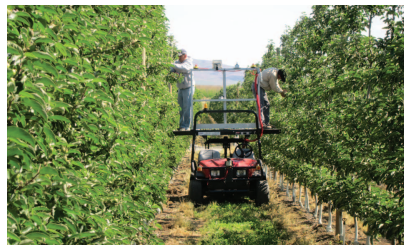
Figure 1. Workers in a commercial orchard conducting green fruit thinning from onboard an autonomous orchard vehicle moving slowly down the row. (Photo courtesy of Carnegie Mellon University, United States.)
