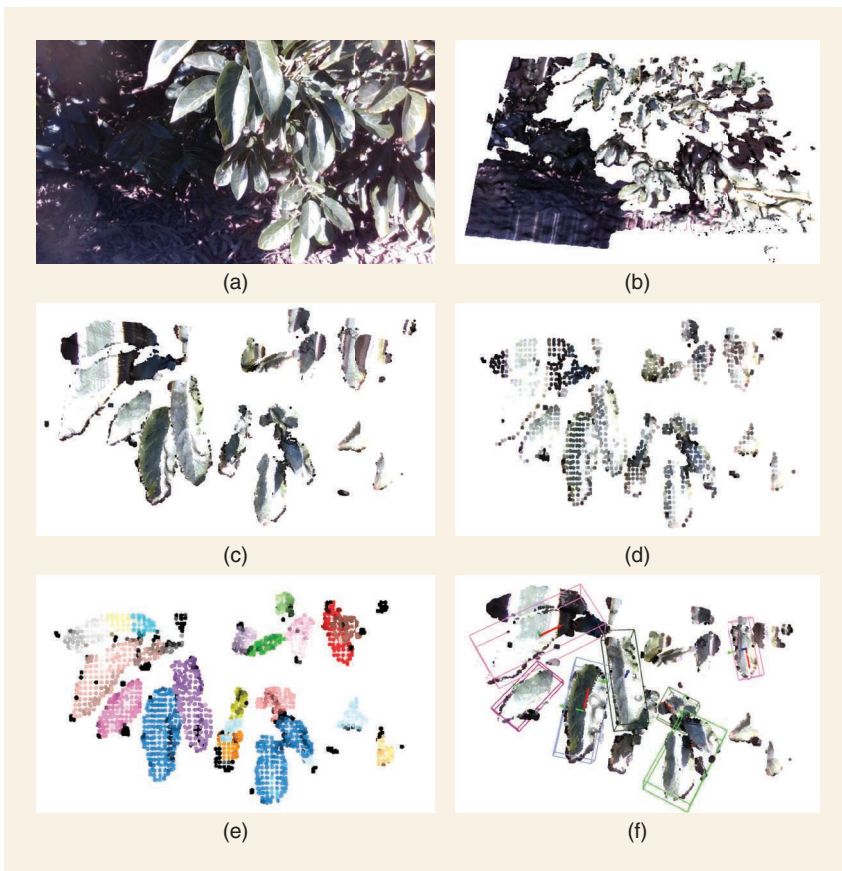
FIGURE 6. Key steps in our proposed leaf detection and localization process. The sample here corresponds to an outdoor point cloud: the (a) corresponding RGB image of the tree, (b) raw point cloud, (c) background removal, (d) downsampled point cloud, (e) segmented clusters, and (f) detected candidate leaves without 6D pose bounding boxes. (Image taken from [3].)
