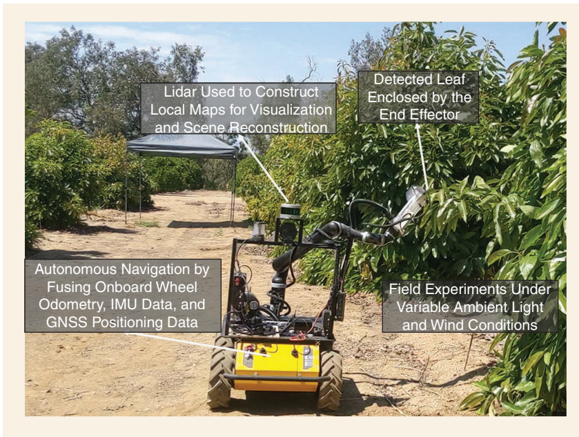
FIGURE 3. The agricultural robot used in this work for robotic assessment of a crop’s need for watering. IMU: inertial measurement unit; GNSS: global navigation satellite system.
