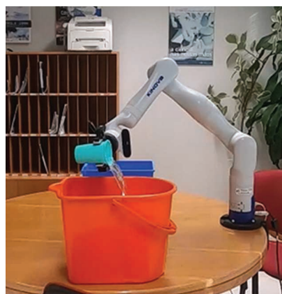
FIGURE 2. The robot understands the object’s physical properties and selects the most appropriate kinematics and manipulation action. Details are provided in [5]. (Source: Photo by Linda Lastrico, IIT; used with permission.)
