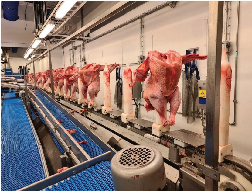
FIGURE 4. An example of an assistive system used in Norway, which presents turkeys on a moving conveyor system for skilled operators to cut.
