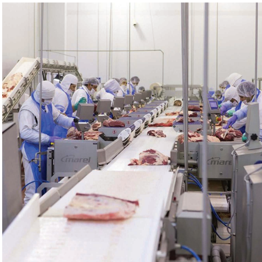
FIGURE 3. A conveyor system combined with sorting stations (Marel, StreamLine) where performance of individual operators can be monitored, and tasks allocated automatically.
