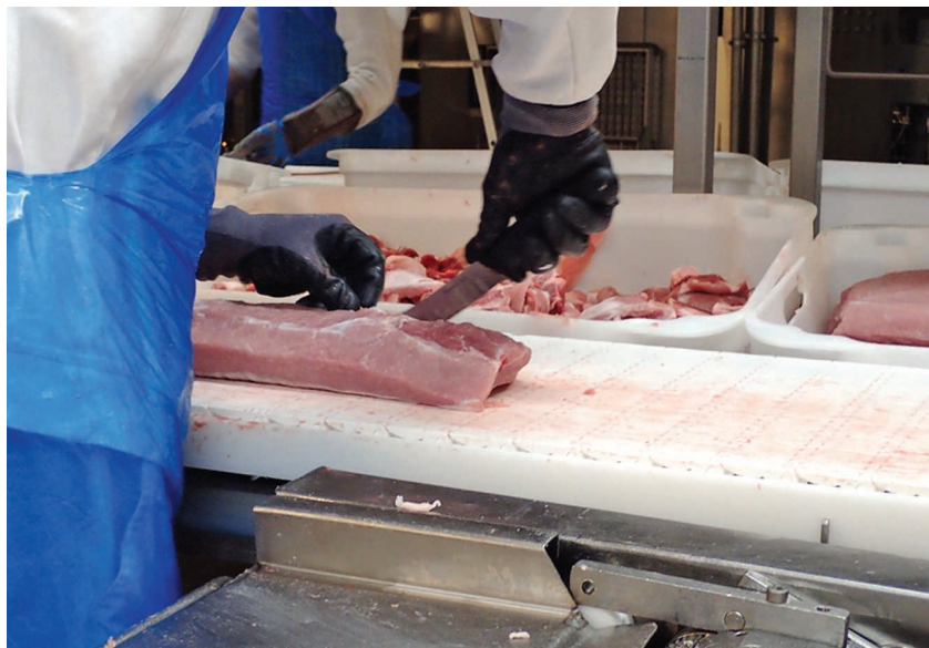
FIGURE 2. A conveyor system in a small processing plant, where butchers are cutting and trimming pork loins. For small processors, the workflow typically includes fewer automatic solutions, relying much more on manual labor.
