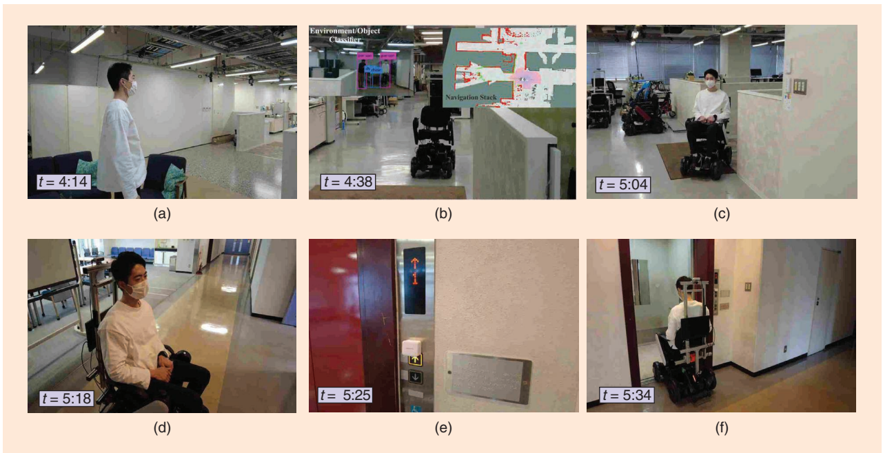
FIGURE 11. The outdoor scene. (a) The user desires to go out and requests the global intelligence via voice command. (b) Based on the user's data and health preferences, a wheelchair robot is selected and it approaches the user autonomously. (c) The wheelchair navigates to outside facility. (d) The user calls for the elevator. (e) Smart switches are actuated and the elevator button is called. (f) The patient takes control of the robot with shared autonomy to move the wheelchair robot.
