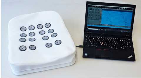
Fig. 1. Multi-channel lung sound recording device.
