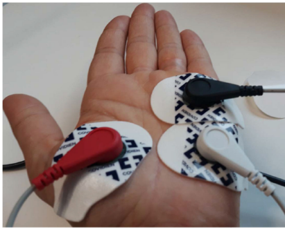
Fig. 2. Placement of the electrodes during proof-of-concept measurements; two current-carrying (CC) electrodes (white, red) and one pick-up (PU) electrode (black).
