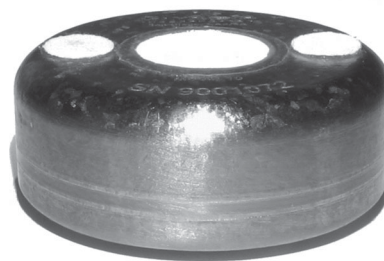
Fig. 1. Glucose sensor/telemetry system implant [9]. The implant is 3.4 cm in diameter and 1.5 cm thick.
