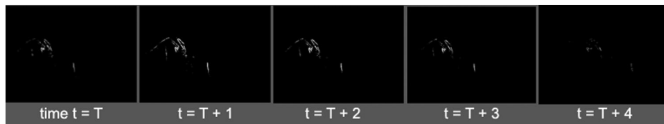
Fig. 2. Sample activity map generated using PLIM, illustrated across a breathing cycle. The subject's breathing is detected around the edge of the subject and folds in the bed clothes. The activity level grows and falls in a cyclical manner through the breathing cycle.
