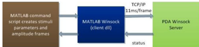
Fig. 8. Device connectivity and data exchange in an offline mode.
