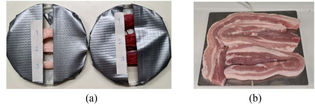
Fig. 2. Ex vivo animal tissues used in the experiments, with specific details provided in Section II-C. In the image (a), three sections of porcine adipose tissue (on the left) and muscle tissue (on the right) are presented. These tissue samples were employed for diffuse reflectance spectroscopy (DRS) measurements and were secured onto the plate using gray tapes. In image (b), the representation features the porcine tissue that underwent electrosurgery.
