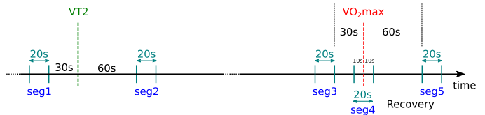
Fig. 8. Position in time through the maximal exercise test of the five 20-second segments extracted from the full ECG of each subject. The numbers of the segments are sorted in time in ascending order. The first segment was extracted 30s before VT2 and corresponds to heavy intensity; the second 60s after VT2 (severe intensity); the third 30s before VO_2 max (highly severe intensity up to exhaustion); the fourth at the moment of exhaustion (centered in VO_2 max); the fifth 60s post-exercise, i.e. during the recovery after exhaustion.
