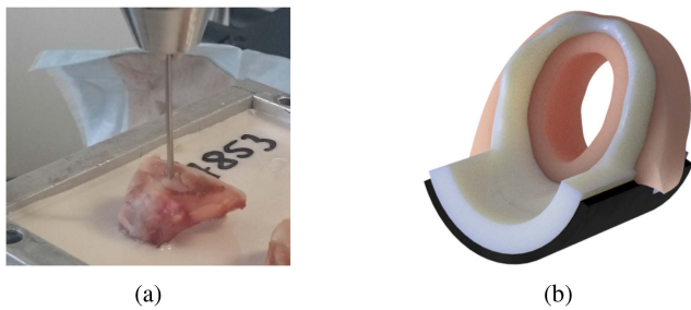
Fig. 2. Cricoid cartilage and surrounding tissue - real cricoid of a human versus artificial, simplified replica; (a) measuring forces while penetrating cricoid cartilage, (b) rendering of an artificial, simplified cricoid cartilage (white) with soft tissue (pink) and sensor mat (“Smart Artificial Soft Tissue,” black) underneath (soft tissue partially removed to reveal cartilage).
