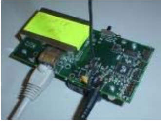
Fig. 2. Crossbow MIB600 “emote” interface board. Attached to a Mica2 or MicaZ “mote”, provides remote reprogramming and data logging capabilities.
