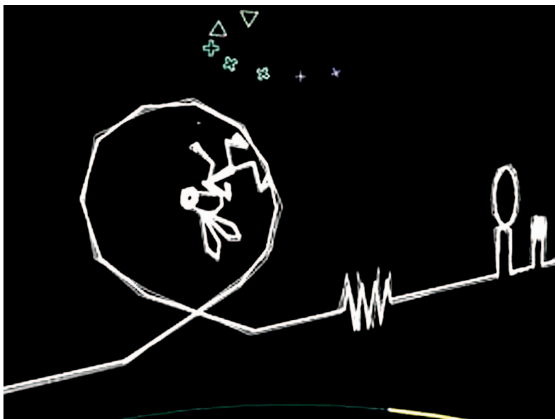
Figure 2. Vib Ribbon by NaNaOn-Sha and Sony used minimalist vector graphics. This allowed the entire game to be cached into memory while retaining a distinctive look.
