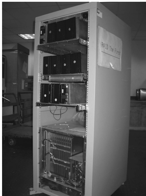
Figure 2. First-generation Berkeley RAID prototype, with RAID 5 functionality implemented across 32 disk drives. A larger second-generation prototype with 192 disk drives is on display at the Computer History Museum.
