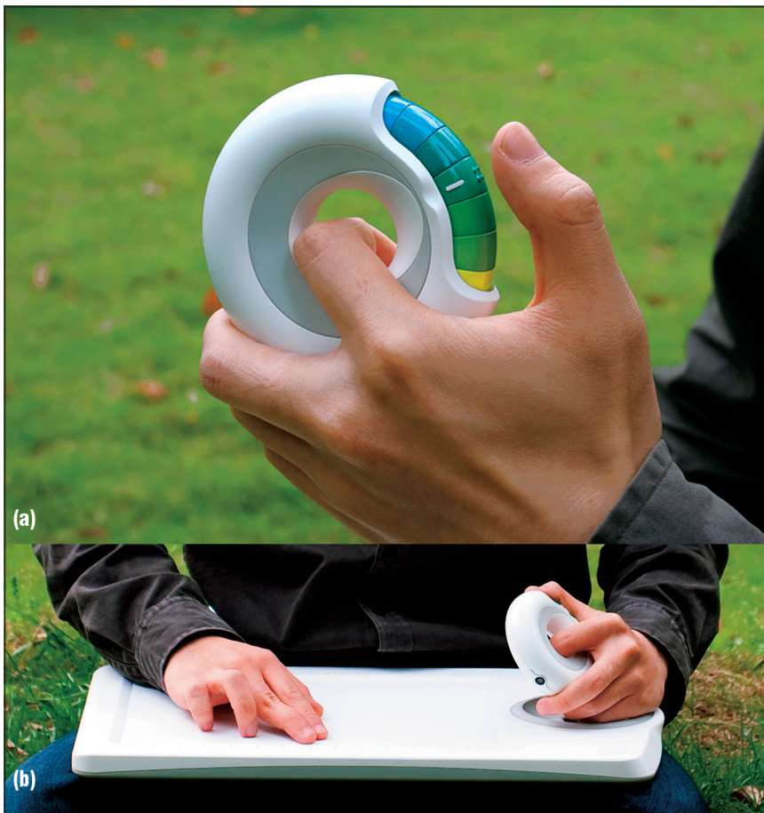
Figure 1. Touch Color's (a) color wheel and (b) tablet work in concert to let users feel the heat of colors in an image.
