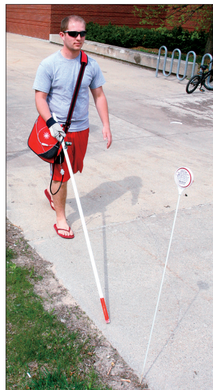
Figure 2. The Smart Cane and a miniature navigational system inside the bag work together to detect RFID tags on mini flags sticking out of the ground. (Source: Robert Barclay; used with permission.)
