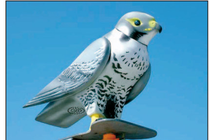
Figure 2. The Robop robotic scarecrow resembles a peregrine falcon and scares away pest birds.
