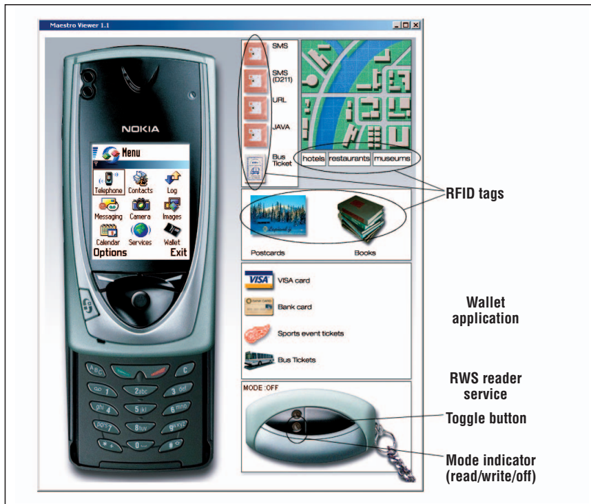
Figure 3. The RFID read-write-send virtual prototype as seen on a PC screen: on the left, a functional simulation of a mobile phone; on the right, the user interface of the RFID RWS prototype.
