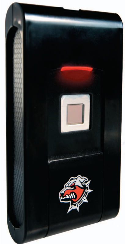
Figure 6. Realm Systems' BlackDog self-contained personal server.
