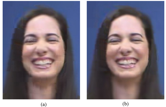
Fig. 9. Kristen and Sara sequence coded in low-delay B configuration at QP37. (a) Deblocking turned off. (b) Deblocking turned on.
