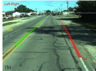
Fig. 12. (a) Categorization of labels based on compatibility with the mother line (plotted in purple): compatible labels at the left (green), right (red), far left (yellow), or far right (cyan) of the mother line. (b) and (c) Final results plotted on the input image and bird's eye view map. Green: close line at the left. Red: close line at the right. Yellow: far line at the left. SYSY: double solid yellow. SW: (single) solid white.
