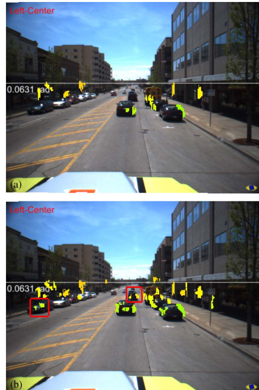
Fig. 8. Detection improvements using multiple layers. (a) Obstacles identified using a single layer. (b) Same frame processed using three layers, with some of the differences circled in red.
