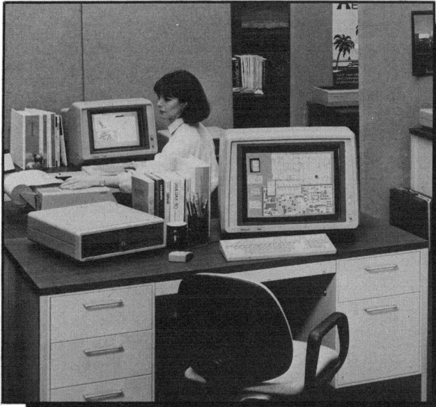
Figure 6. In August 1984, Tektronix introduced the 4404 AI System and, in August 1985, the 4405 and 4406 AI Systems at about $12,000, $15,000, and $24,000. The three products feature the Smalltalk-80 programming environment. Tek Common Lisp, Franz Lisp, or MProlog are available as options.
