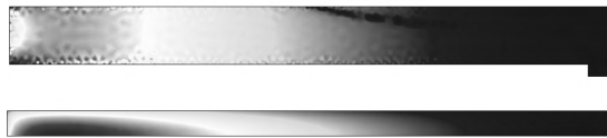
Fig. 8. Flow simulation using 3D gauge solver. Top: shear rate in the gap; bottom: pressure on the lateral face.
