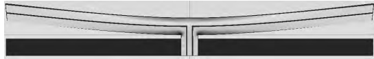
Fig. 3. Top-view of driving/sensing mode at 37658 Hz; also shown the surface charge density on top of the ZnO layer.
