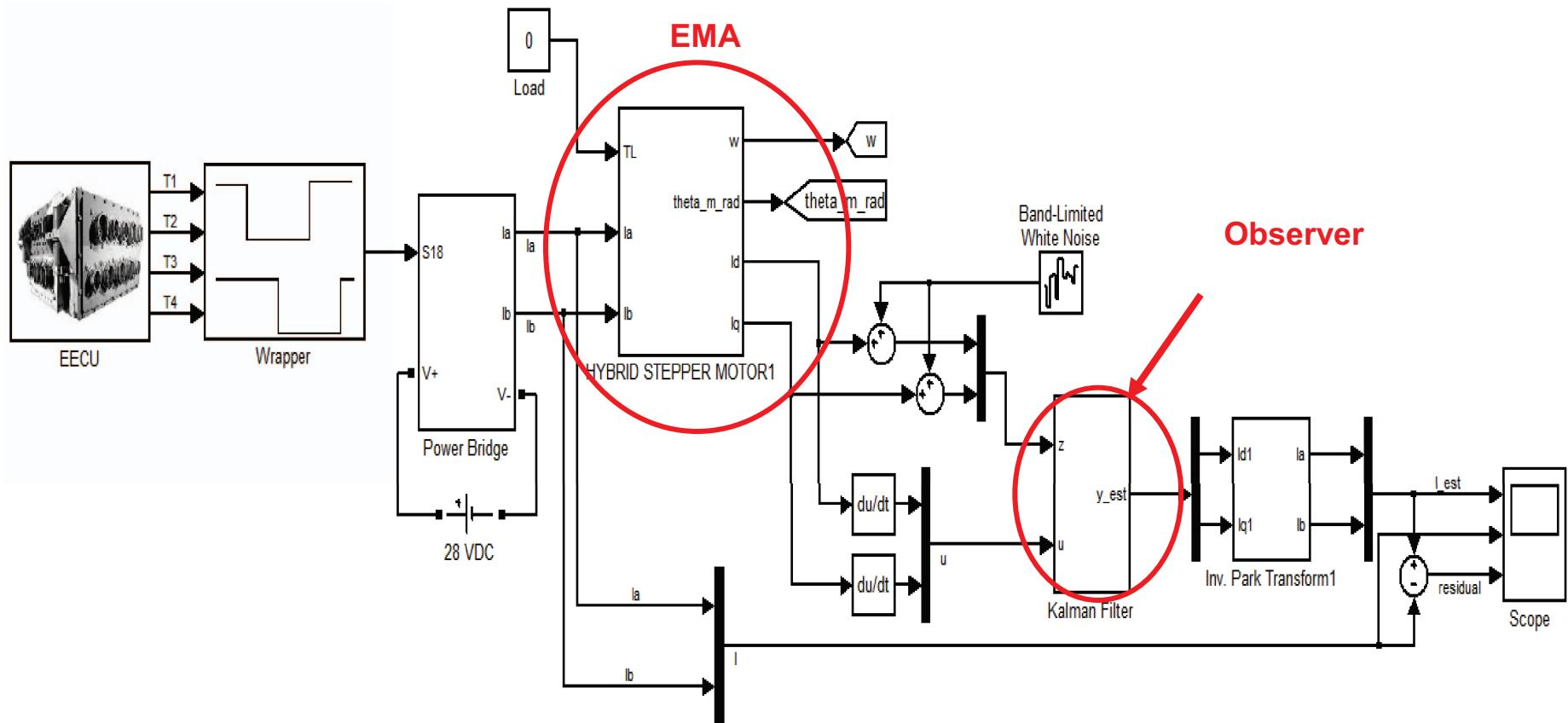
The HSM Model is linearised to fit with a Standard Kalman Filter
