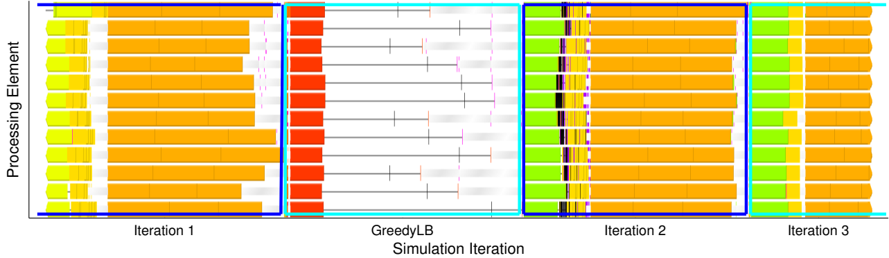
Figure 13. Effect of Load Balancing: heavily imbalanced in Iteration-1 (three PEs have more load than the others). GreedyLB at the start of second iteration reallocates chores to processes with lighter loads. Iteration-2 shows better load distribution.
