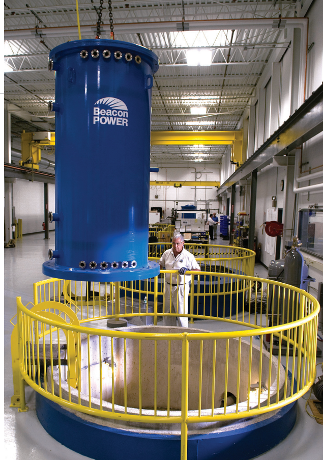
REVVED UP: A flywheel generator is lowered for high-speed tests. PHOTO: BEACON POWER CORP.
