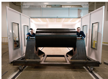
DRUMROLL, PLEASE: A carbon-fiber flywheel is removed from a coating chamber. PHOTO: BEACON POWER CORP.
