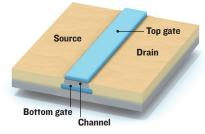
PRESENT, FUTURE, AND FUTURE: Today's CMOS transistor is planar, but chip makers are exploring more power-efficient threedimensional structures (FinFET) as well as a planar structure with two gates. Technologies' principal scientist for CMOS devices Klaus Schrüfer, multigate technology is a game changer: "Multigate is the only device architecture for scaling" into the foreseeable future, he says.
