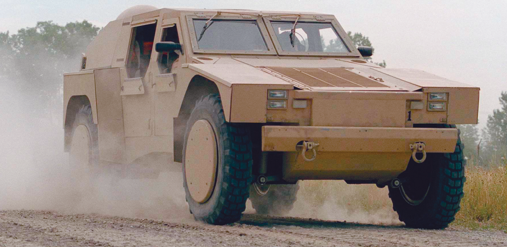
SHADOW: Meant to be stealthy as well as fuel-efficient, this armored vehicle being developed for the Pentagon would have a hybrid drivetrain, combining a combustion engine and battery-powered traction.
