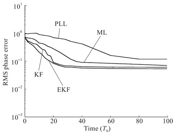
Fig. 5 RMS phase error for Rayleigh channel
