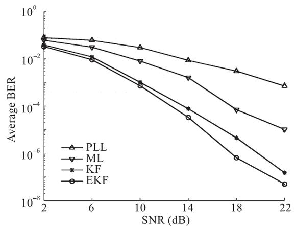
Fig. 4 Average BER versus SNR for AWGN channel
