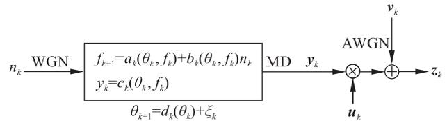
**Fig. 1 Discrete-time model of a digital communication system**
