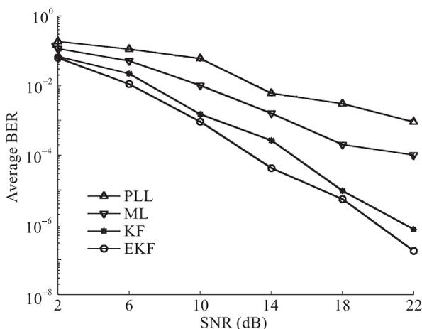
Fig. 6 Average BER versus SNR for Rayleigh channel
