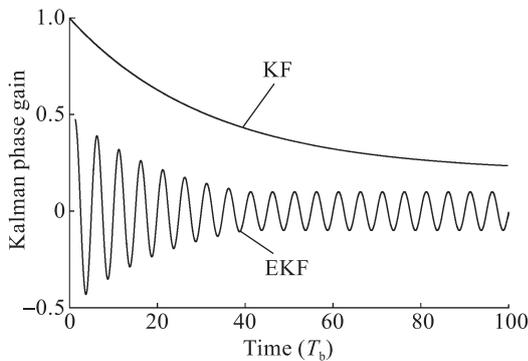
Fig. 2 Pre-computed Kalman phase gains for the KF and EKF schemes
